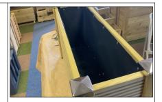
Next comes the lining, take the small roll of liner and place it in the bottom, it might be a little fiddly and it might help to cut the corners to get them flat. (15mm large flange screws) Put in 2 screws in the middle and one in each corner.
