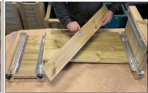
Now comes the screwing, use the 3.5 x 25 mm screws, you want to screw in the bottom piece first using the bottom holes in the metal and then the top piece. After that place in more screws, put in 2 screws per plank for each side, try and place one at the bottom of the plank and one at the top, now the holes in the metal can be random so it doesn't matter to much if you need to use the next hole down.
